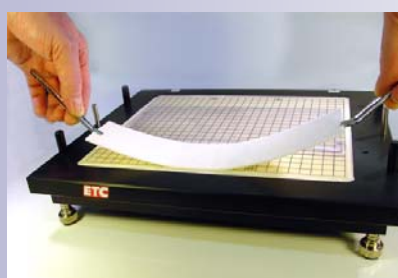
Applying the electrode wicks onto the gel-edges
