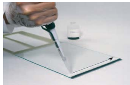
Fig. 2: Pipetting dist. water along the spacer of the closing side
