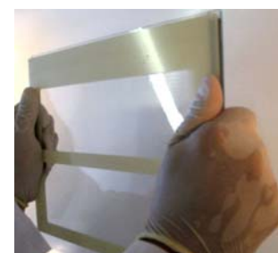
Fig. 6: Close the cassette, press tightly.
